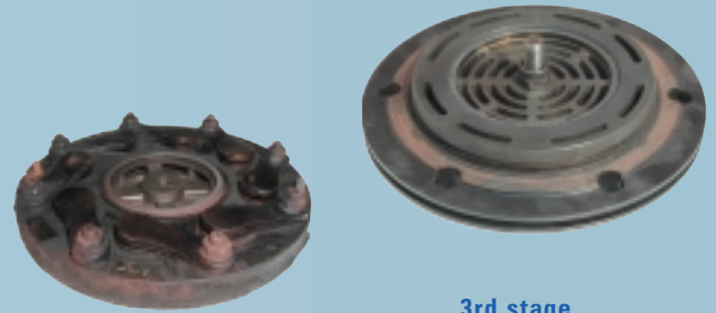
3rd stage air-cooled valve after 2.500 hours
